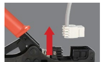
Step 4 – Release the handle and remove the terminated jack!
